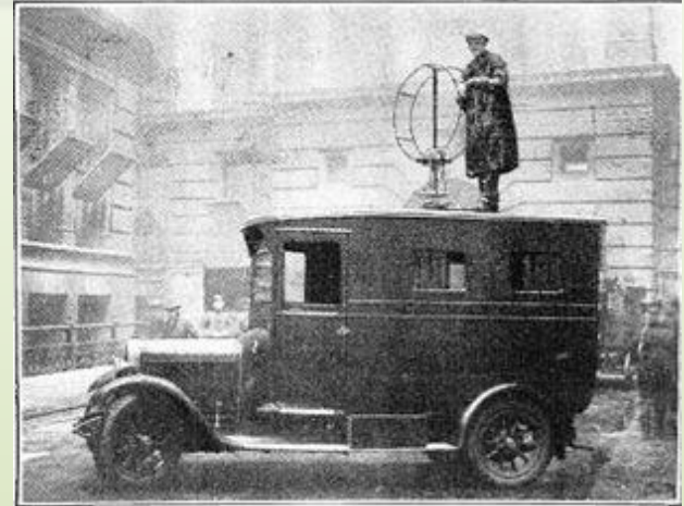
British Post Office RDF lorry from 1927 for finding unlicensed amateur radio transmitters.
