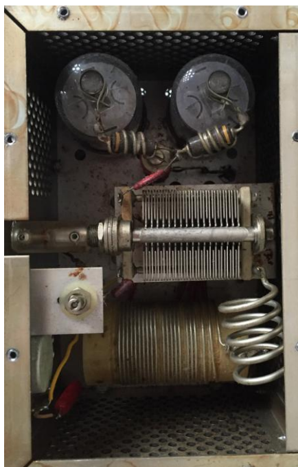
Power Amplifier Compartment in the back left corner of the top chassis. (Front Panel is to the left.)
