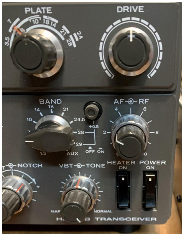
Radio shows both power switches “ON” and AF Gain at about 30% level
