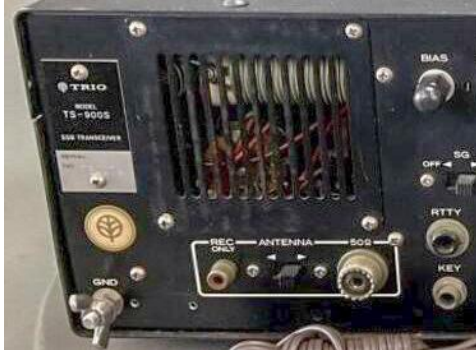
Rear Left View of the TS-900X Shows air escape grill from blower. Schulman Auction Photo
