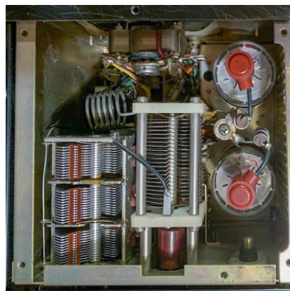
Trio (Kenwood) TS-900 HF Transceiver PA Compartment. This is a top view with the Front Panel toward the bottom of the picture.
