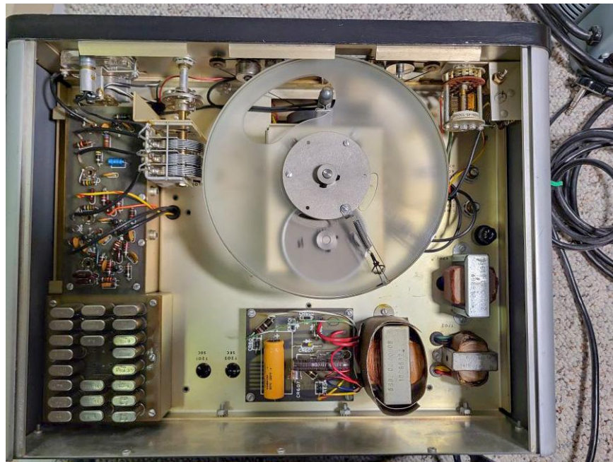
Bottom View – Hammarlund HQ-225 at K9OA – Front Panel at Top. Note Mu-Metal shield material wrapped around the power transformer that is to the right of the Power Supply board.
