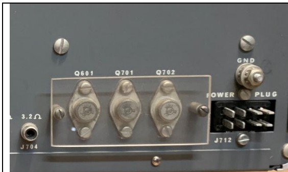
This view shows the lower right-hand corner of the HQ-215 Rear Panel. Note the Cinch-Jones Power Plug, the Ground Lug, the External Speaker Connector, and the three sheet Plexiglas™ isolated power transistors. Transistor Q601 is the radio's Power Supply Pass Transistor. All three transistors are RCA 40310 devices. W9MXQ
