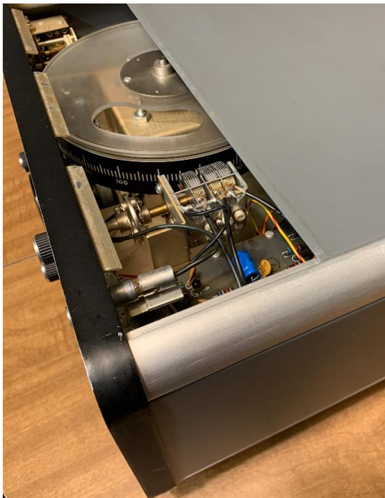
Hammarlund HQ-215 Receiver Right Front Corner view with the Top Cover pulled back a few inches. See how the Panel slides into the right upper extrusion.
