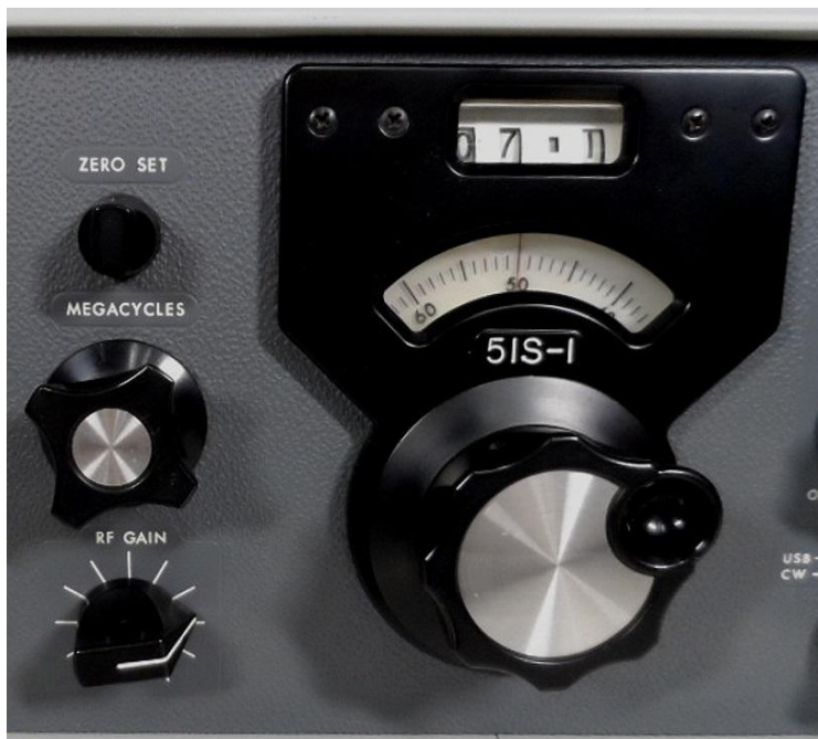
Collins 51S-1 Receiver Tuning, Band Set / MHz Dial, and Bandswitch (MEGACYCLES) W9MXQ – 51S-1 Service Manual
