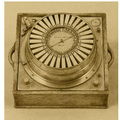
FIGURE 3 – POINTER TELEGRAPHS USED MULTIPLE WIRES
