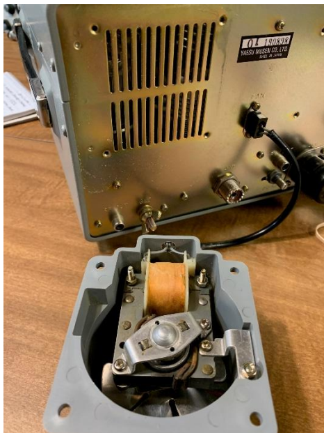
After Cleaning FT-101ZD Rear Panel and Fan Cleaned and Fan Lubricated
