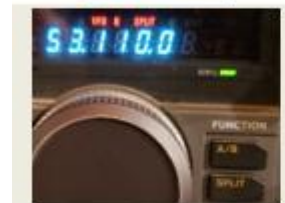
Set First Frequency to 53.110, VFO A preferred (ignore VFO B shown in picture)
