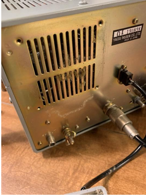
Before Cleaning FT-191ZD Rear Panel Fan Just Removed
