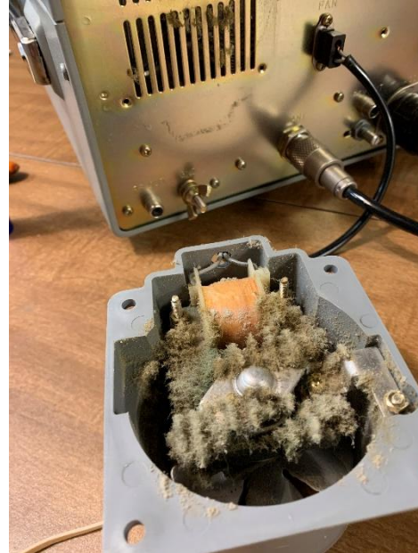
Before Cleaning FT-101ZD Rear Panel and Fan Showing Lint in Fan Assembly
