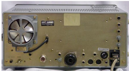
Rear Panel of the FT-101ZD Note Optional Fan is Installed See Tape over DC Module Connector 8 Note Power Connector at Lower Right
