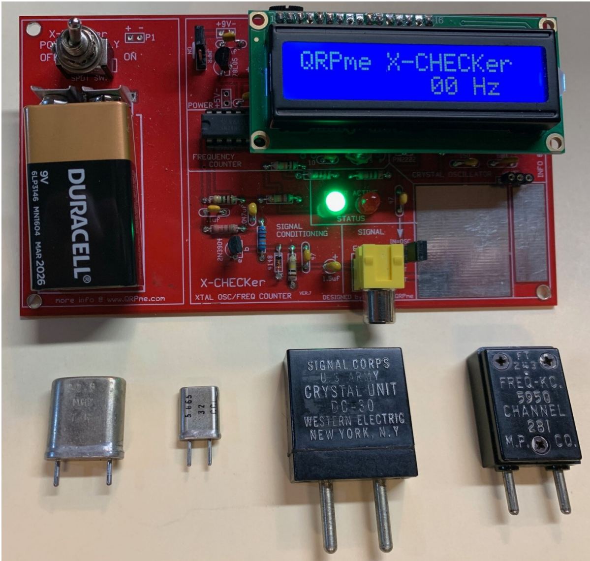
QRPme X-CHECKer Device Readout is indicating it is ready to test a crystal.
